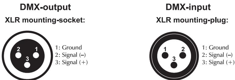
If you are using controllers with this occupation, you can connect the DMX output of the controller directly with the DMX input of the first device in the DMX chain. If you wish to connect DMX controllers with other XLR outputs, you need to use adapter cables.
